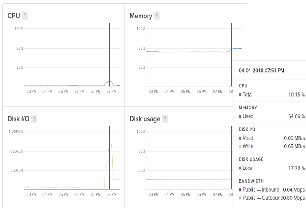
Figure 6.6.1: Server monitoring graphs during continuous and standby web platform operation modes.
